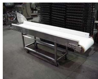
Cross-scrap - belt type, stainless steel slide bed. Standard unit general purpose.
