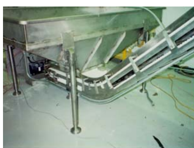
Scrap Conveyor infeed, hopper feed.
