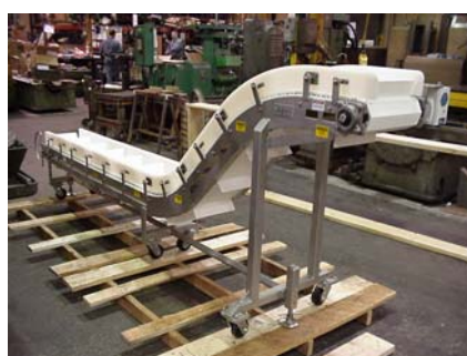
Conveyor Z-type 71- 1/2" long bed.
