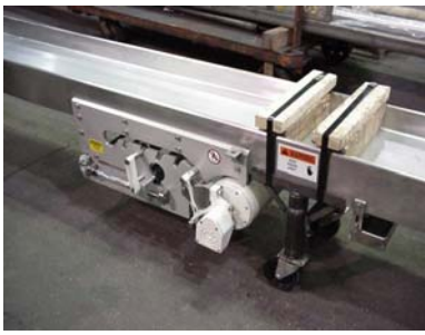
Scrap Conveyor -12" wide belt with modular drive, incorporating drive roller, take-up & sew loop.
