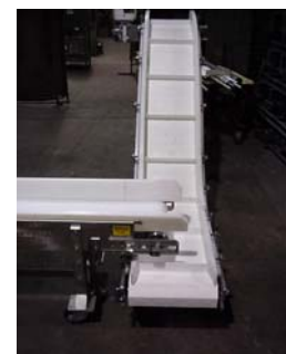
Cross-scrap - Conveyor to Z-type Conveyor.
