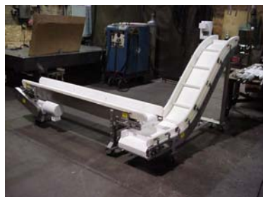
Cross-scrap - belt type, stainless steel slide bed. High sides, bulky product.
