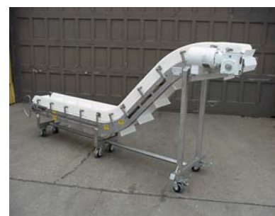
Conveyor Z-type 53- 1/2" long bed.
