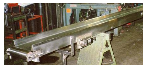
Scrap Conveyor 12" belt, infeed, formed S.S. bed.
