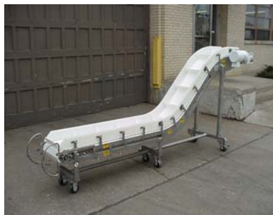
Conveyor Z-type 53- 1/2" long bed.
