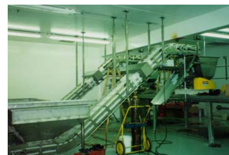
Scrap Conveyor with metal detector.
