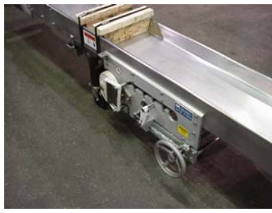
Scrap Conveyor -12" wide belt with modular drive, incorporating drive roller, take-up & sew loop.
