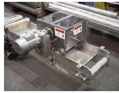
Scrap Conveyor -12" wide belt with scrap cutter.
