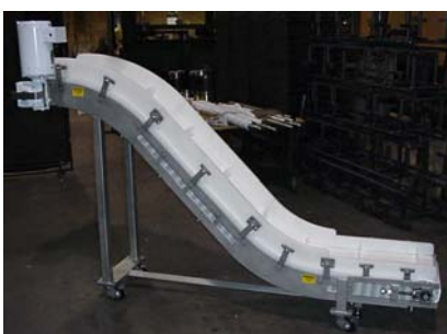
Scrap Conveyor Z-type short (19") bed low profile.
