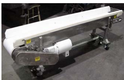
Cross-Scrap, belt type, stainless steel slide bed, chain drive, narrow width.
