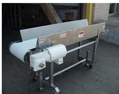
Cross-scrap - belt type, stainless steel slide bed. High sides, bulky product.
