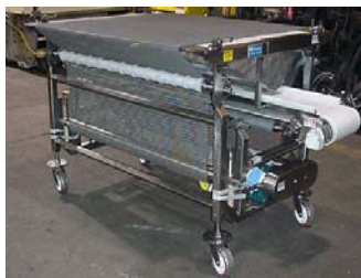
Salt Reclaimer Conveyor, wire mesh with retractable discharge noser.
