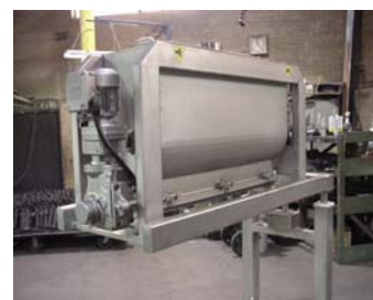
Salt applicator mounted on adjustable height C-Frame
