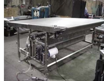
Oven Take-off (Special R&D) with adjustable height in feed - manual with retractable discharge noser..
