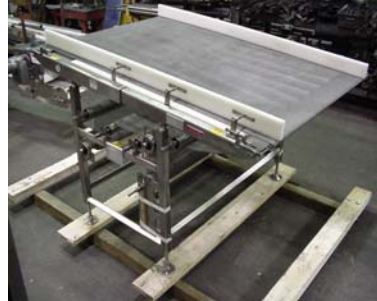
Oven Take-off, standard unit wire mesh 45" wide x 72" long with retractable nose section.
