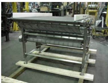
Oven Take-off, standard unit wire mesh 45" wide x 72" long with retractable nose section.
