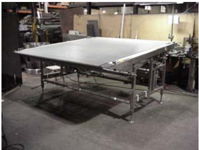
Oven Take-off, wire mesh 87" wide x 108" long with retractable nose section.
