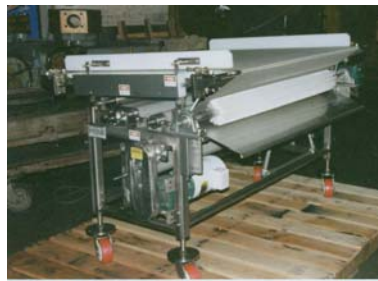
Oven Take-off, Special unit wire mesh 45" wide x 42" long with retractable nose section
