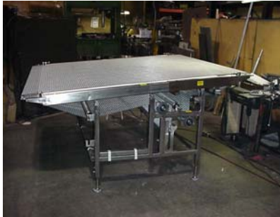
Oven Take-off, wire mesh 87" wide x 108" long with retractable nose section.
