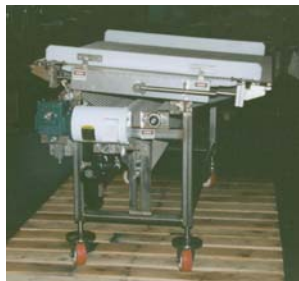
Oven Take-off, Special unit wire mesh 45" wide x 42" long with retractable nose section
