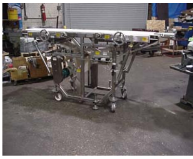
Oven Take-off (Special R&D) with adjustable height in feed & discharge.
