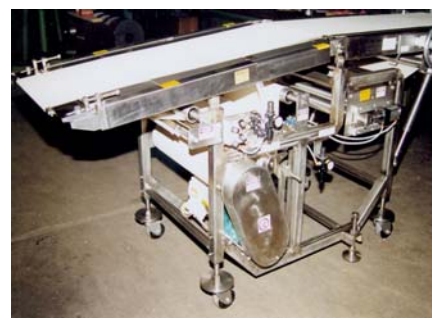
Oven Take-off (Special R&D) with adjustable height in feed - manual with retractable discharge noser..
