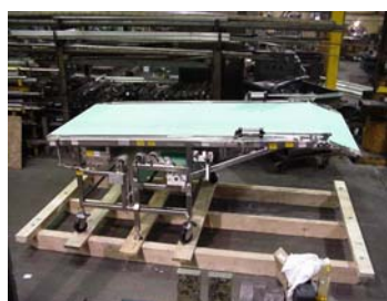
Standard unit 50" belt width x 126" long. The discharge side has a pneumatic lift to prevent heat damage to belt. Infeed features a manual operated dump.
