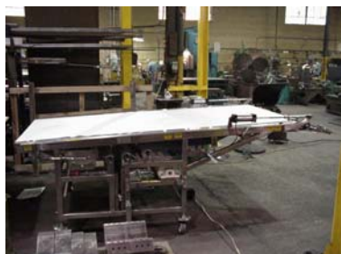
Standard unit 50" belt width x 126" long. The discharge side has a pneumatic lift to prevent heat damage to belt. Infeed features a manual operated dump.
