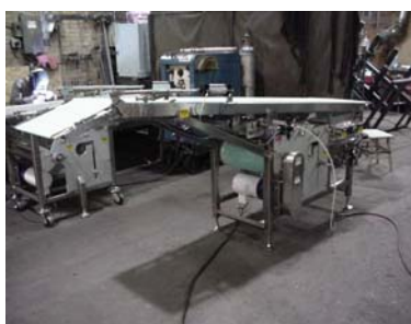
Feed-on, 18" belt x 110" long built for R&D, same features as standard unit
