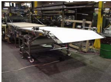
Standard unit 50" belt width x 126" long. The discharge side has a pneumatic lift to prevent heat damage to belt. Infeed features a manual operated dump.
