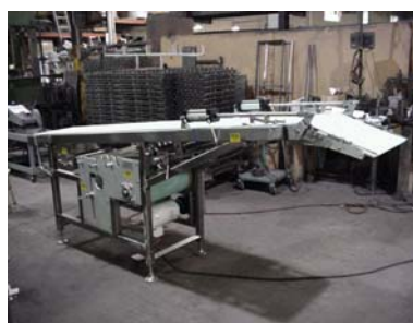
Feed-on, 18" belt x 110" long built for R&D, same features as standard unit
