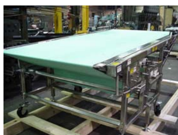
Standard unit 50" belt width x 126" long. The discharge side has a pneumatic lift to prevent heat damage to belt. Infeed features a manual operated dump.
