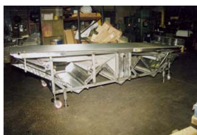
Extended Oil Drain Conveyor, open sides with collection pans. Wire mesh, 42" belt x 192" long.
