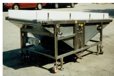
Oil Drain Conveyor, closed sides. Wire mesh, 48" belt x 96" long.
