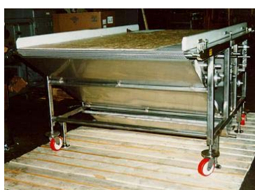
Oil Drain Conveyor, open sides. Wire mesh, 54" belt x 96" long.
