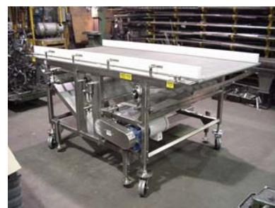
Oil Drain Conveyor, open sides with collection pan. Wire mesh, 42" belt x 96" long.
