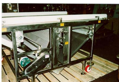
Oil Drain Conveyor, open sides. Wire mesh, 54" belt x 96" long.
