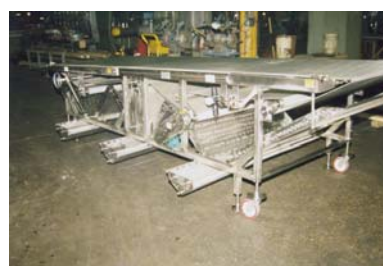
Extended Oil Drain Conveyor, open sides with collection pans. Wire mesh, 42" belt x 192" long.
