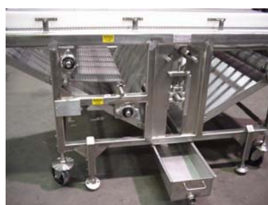
Oil Drain Conveyor, open sides with collection pan. Wire mesh, 42" belt x 96" long.
