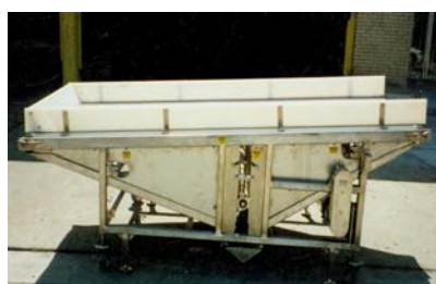
Oil Drain Conveyor, closed sides. Wire mesh, 48" belt x 96" long.
